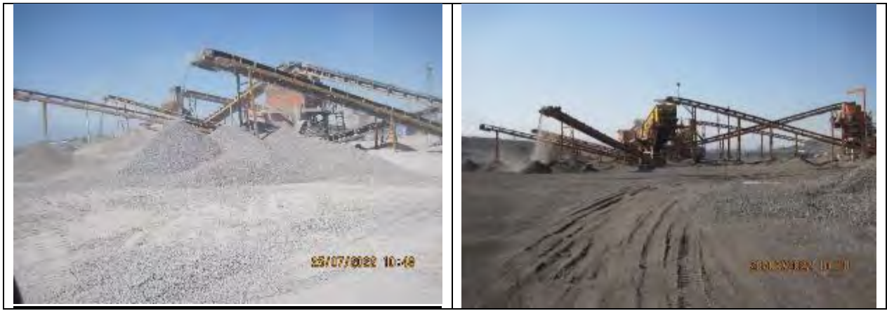
Figure 64 Operation of a stone crushing plant on moistened raw materials
