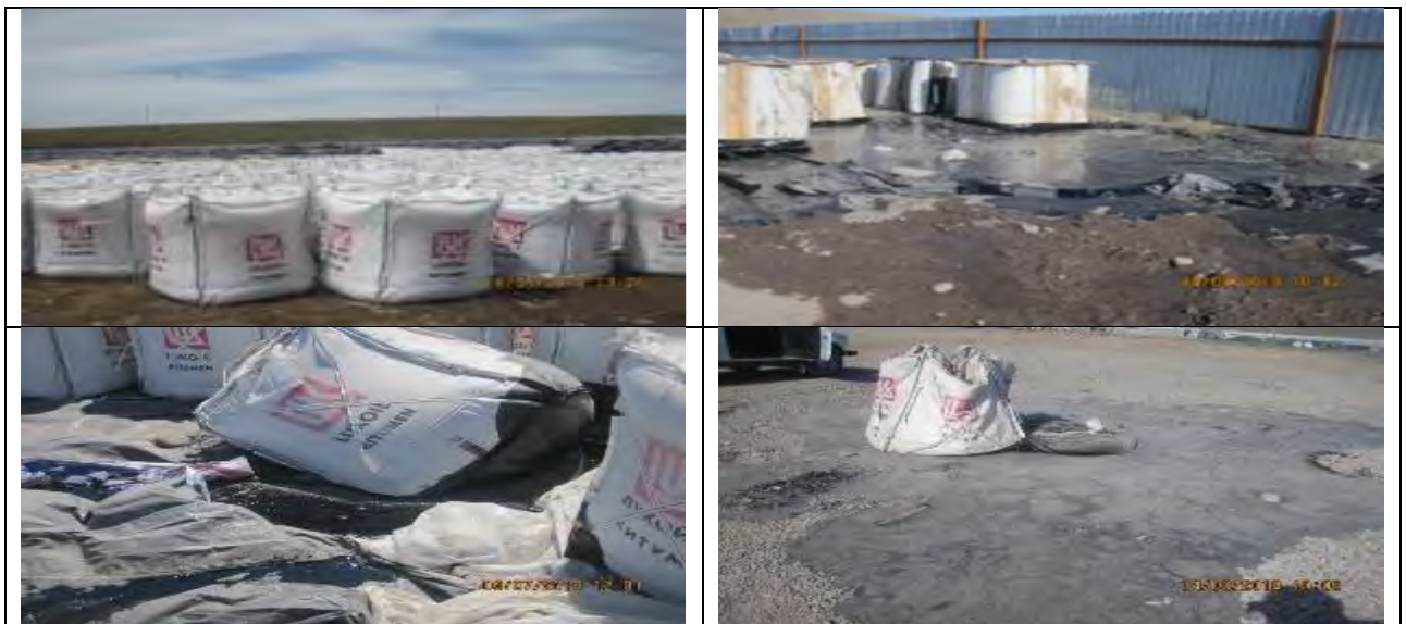
Figure 69 Bitumen in plastic packages. Bitumen leaks to the ground
